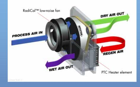
A fan blows air through a porous wheel of Desicant material (water absorbing). The wheel rotates slowly in a housing that provides 3 separate air paths (Main, Regen & Post-cool) through the wheel. As it rotates, all parts of the wheel pass through each air path. In the main path (approx 60% of wheel area) process air passes through the wheel and is dried because the wheel absorbs its moisture, this air is then routed to the 'Dry-Air-Out' duct.
